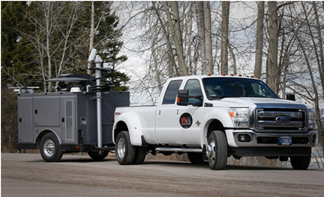
Figure 3-11: Trailer/Towed BBDS Unit [7]
