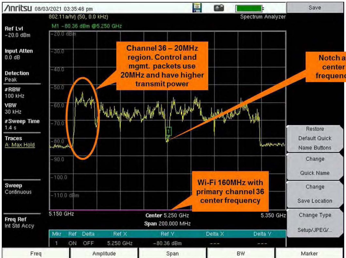
Figure 4. Spectrum Analyzer Frequency Domain FFT Plot of 160 MHz Wi-Fi Signal
