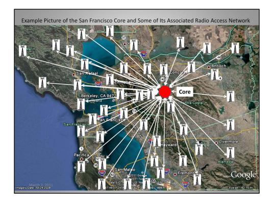
This slide shows what could be the initial buildout of only the San Francisco Core and its associated Radio Access Network (RAN).
