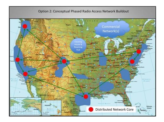
This slide shows a connection between a nationwide Public Safety network and a commercial network through a Clearing House & Roaming Hub.
