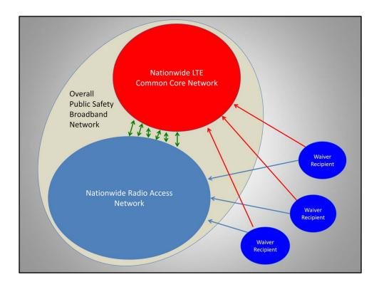
This diagram shows that current/planned investments in Cores and RAN can be gracefully migrated forward from individual cores/RANS operated by Waiver Recipients to a single national network, hopefully leaving minimal stranded investment.
