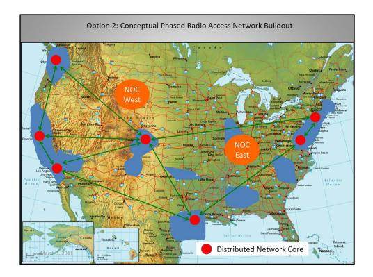
This diagram shows how Network Operations Centers could be geographically dispersed for redundancy and to meet operational requirements.
