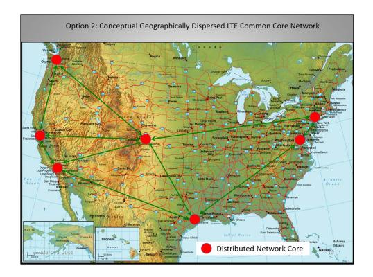
IMPORTANT NOTE: The following slides for Option 2 are conceptual, with distributed core locations based upon geographical separation and population centers. A detailed engineering analysis will be required to determine the proper network topology and appropriate number/placement of primary and hot standby core nodes.
