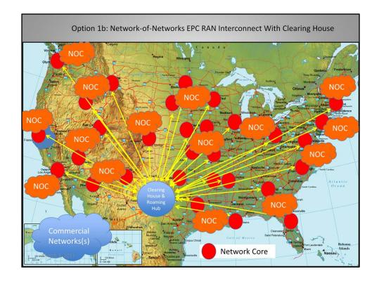
Option 1b employs a Clearing House and Roaming Hub to provide connectivity between Public Safety cores and to Commercial Network(s) to eliminate the myriad of direct connections between each network, but does not address the potentially large number of NOCs required to support the various networks.
