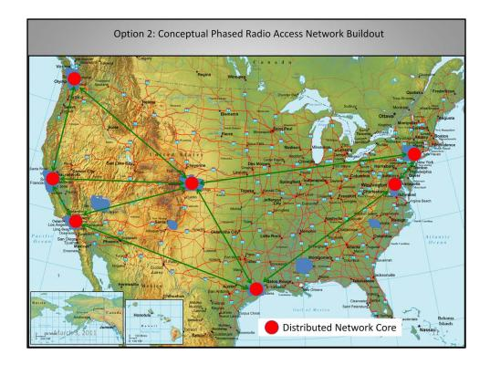
A local core is not required to support diverse geographical areas, as shown by the blue areas that are remote from any of the 7 cores.
